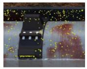
ZERUST® Zerion™ FVS combines VCI and SCI; SCIs neutralize contaminants in liquid, while VCIs protect the vapor space.
